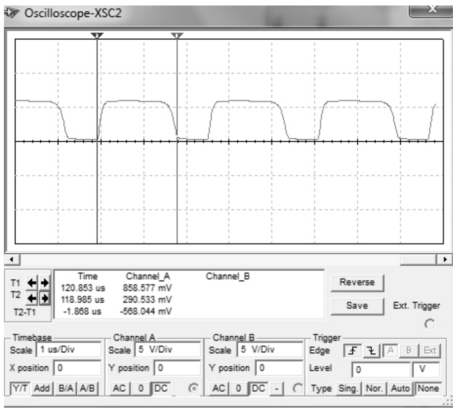
Figure 4: Output waveform for the circuit in figure with inductor coil of 3200uH.
